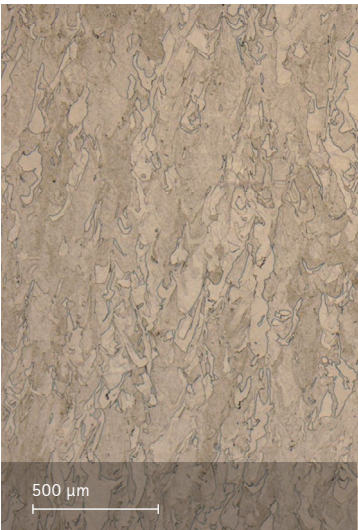
Microstructure solution annealed Etched with etchant Kallings 2
