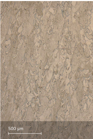
Microstructure solution annealed Etched with etchant Kallings 2
